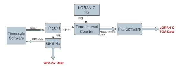
FIG.2 Hardware Configuration at Each Site
