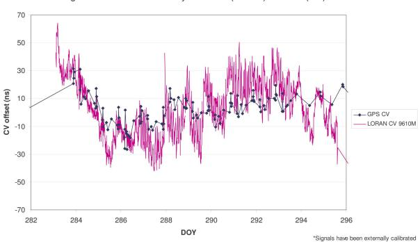
Comparison of GPS Common View vs LORAN Common View\* Long Common View Baseline - Symmetricom (Boulder) to Gillette (WY)
