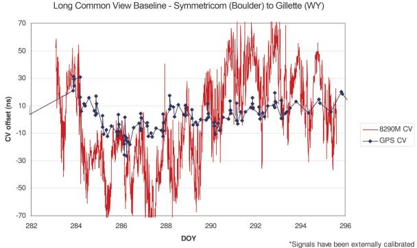
GPS Common View vs LORAN Common View\*
