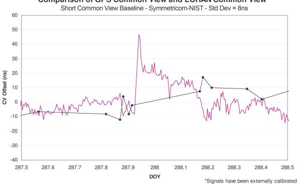
Comparison of GPS Common View and LORAN Common View\*
