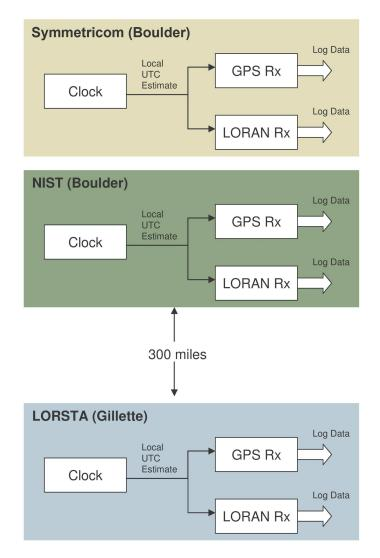
FIG.1 Experiment set-up for Common-View LORAN-C Experiment
